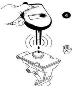
The display will then alternate between the measured boiling point and the recommended minimum for DOT4 and DOT5.1 fluids.
