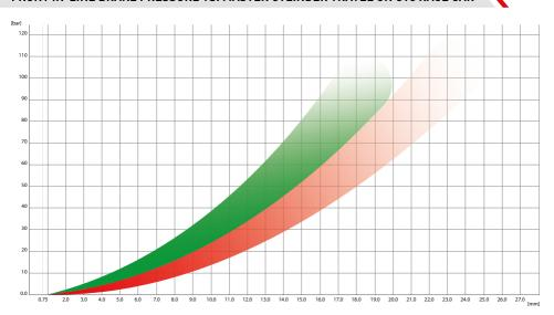
GREEN: New Brake Pads with 29.0 mm averange thickness / RED: Same Brake Pads with 25.0 mm averange thickness
